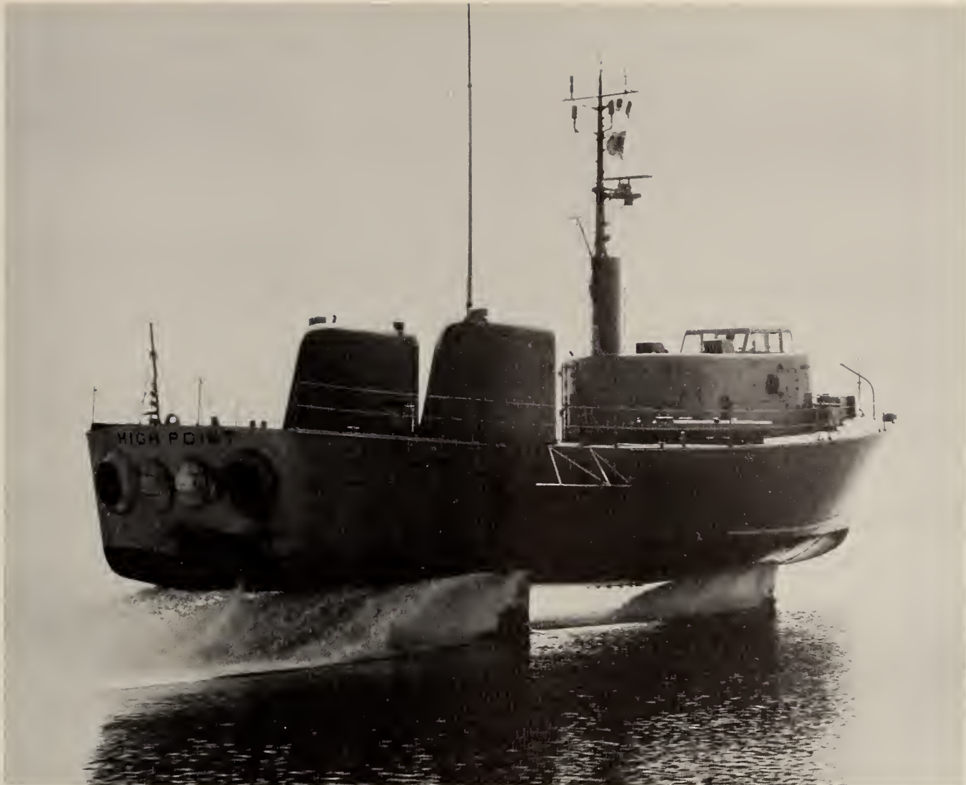
High Point, the U.S. Navy's first operational hydrofoil, is the largest craft of its kind using a wholly submerged foil system. It was built for the Bureau of ships under contract by Boeing.
